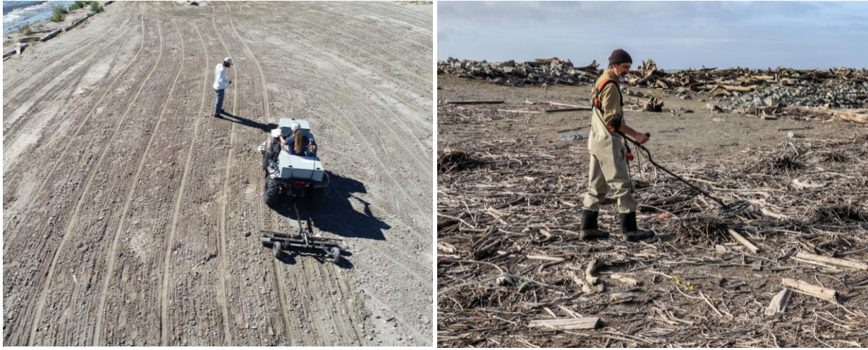
Figure 1. PIT tag detection equipment used on East Sand Island in 2018 which included an eight-coil flat-plate antenna with tow-behind sweep magnet attached to an ATV for use on the Caspian tern colony (left) and hand-held portable antenna systems (right) for use the double-crested cormorant colony and areas not accessible to the ATV on the Caspian tern colony.
